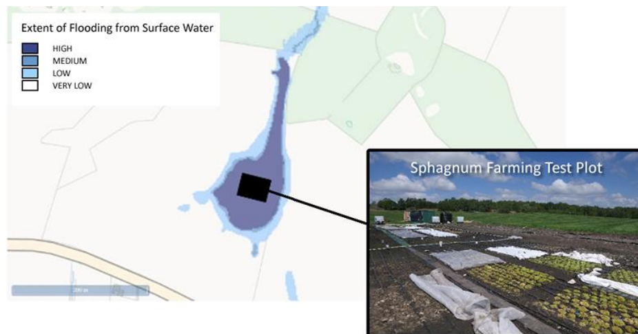
Figure 2.2 Extract from Environment Agency Flood Risk Map for surface flooding, indicating direct correspondence between high-medium risk of surface-water flooding and the locality of former deep peat (now shallow organo-mineral) soil used as test-bed for Sphagnum farming paludiculture with irrigation from above.
